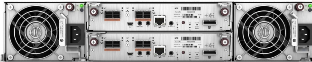
Figure 19. HPE MSA 2052 (rear facing, dual controllers)
