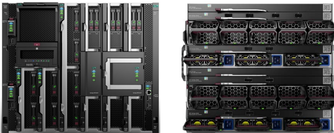
Figure 2. Front view and rear view of HPE Synergy showcasing composable infrastructure appliances
