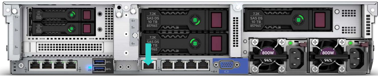
Figure 7. Rear view of example HPE ProLiant DL380 Gen10 server highlighting iLO5 port
